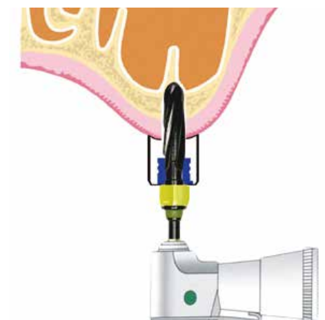
Fig 18. Dome-shaped crestal approach bur under the septum
