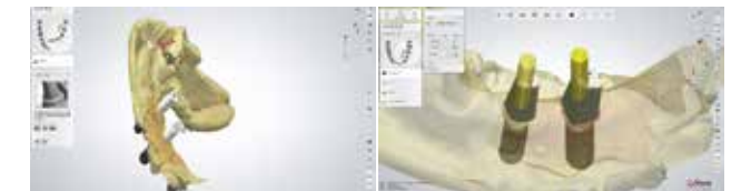
[Figure 21] Designing Ti Customized Abutments and PMMA Provisional Crowns
