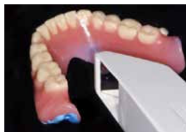
③ Scan teeth and both of interior/ area where the marker is attached.
